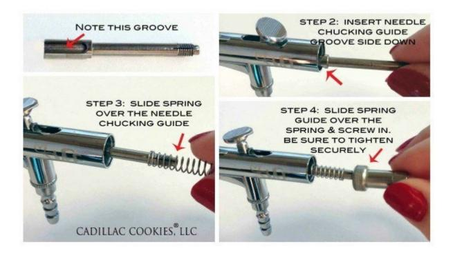
After you've replaced and tightened the spring guide (Step 4), double check your trigger. Pull it back and make sure it's not too loose. If it feels too loose, then you've not tightened the spring guide enough.
